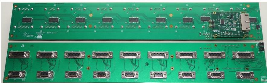
Some OEMs have built backplane boards to handle decoding, interconnections and interfacing using ribbon cables to connect to the interface board. However there are reliability issues with ribbon cables, especially in military or other high-reliability systems. The Modular System Controls approach is to use distributed processing. A small module about the size of a credit card containing a low cost
